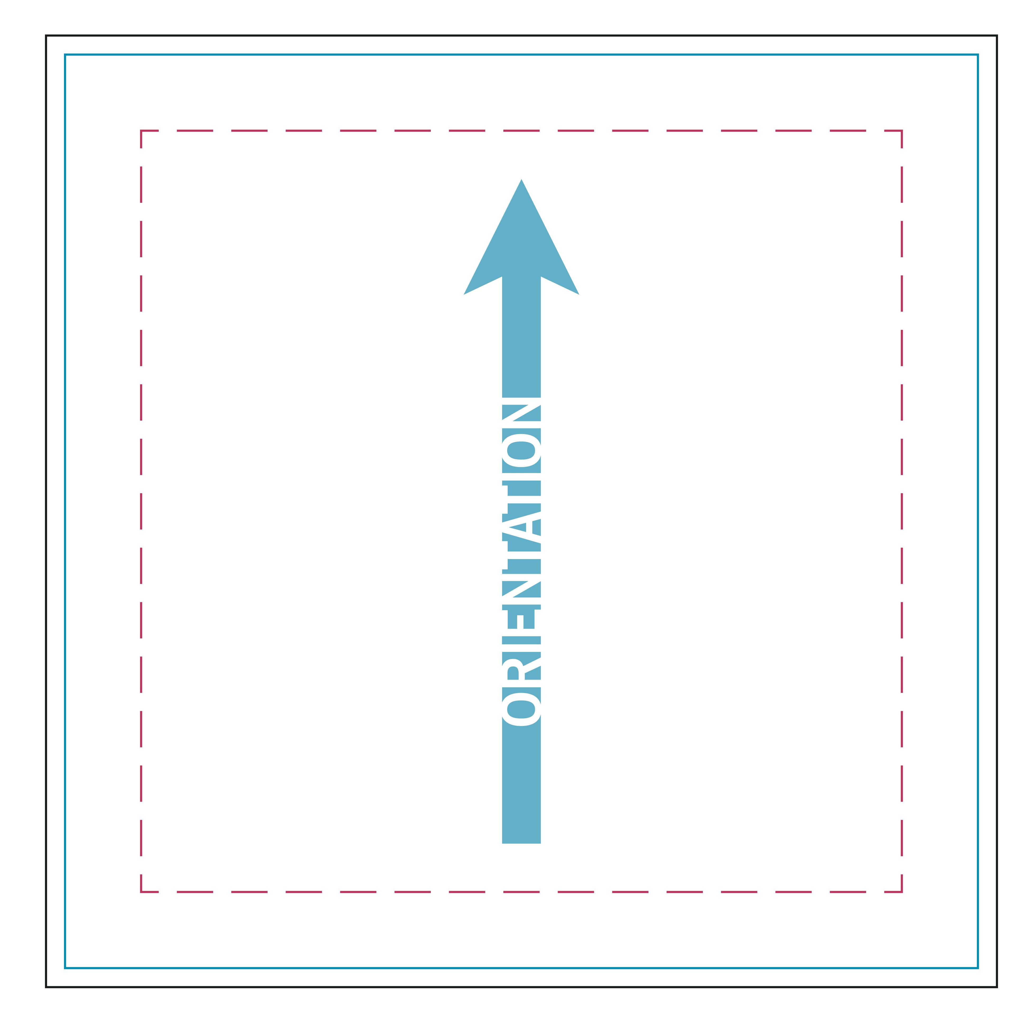
X-FACTOR: A term describing the result of tension at all corners and connection points of an Xpressions skin when placed on a frame. The artwork will be stretched with the least amount of distortion at the center of each quad, and the most distortion within the outer 3-5" of the skin. It is not a live area, as the image will be visible.
