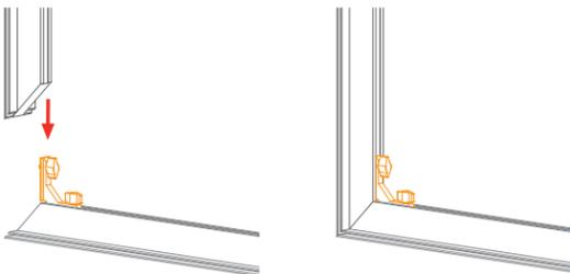
Keep corner connectors attached to horizontal extrusions.
