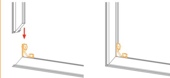
Keep corner connectors attached to horizontal extrusions.
