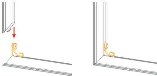
Keep corner connectors attached to horizontal extrusions.
