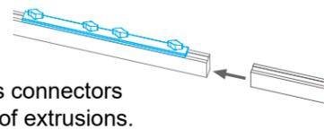
2. Slide tool-less connectors across seam of extrusions.
