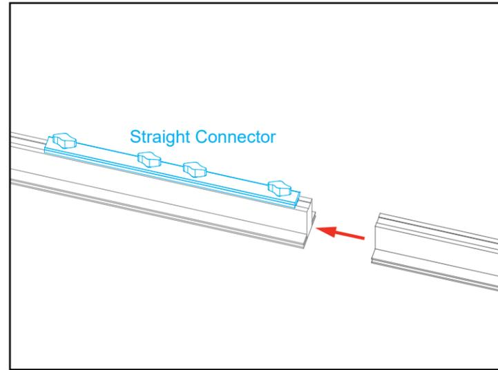
Slide connector across seam of extrusions.
