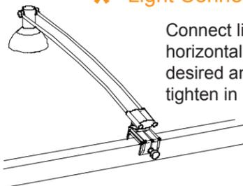
Connect light to horizontal where desired and tighten in place.
