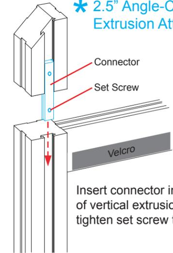
Insert connector into groove of vertical extrusion, then tighten set screw to secure.
